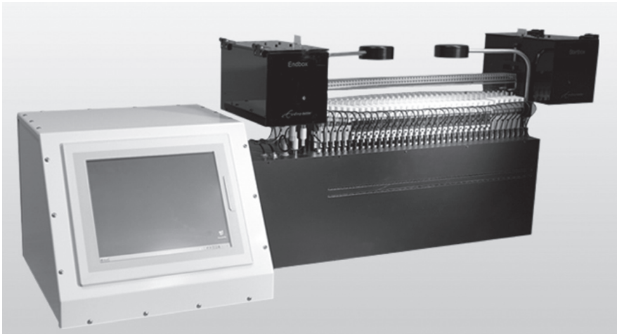
The Erasmussladder Version 2; left: the real-time computer, right: the sensors and electronics
