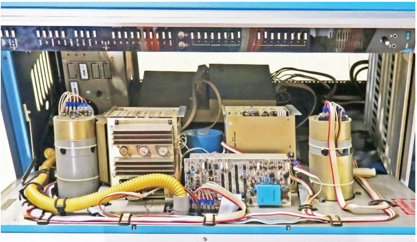
*Figure 8: Inside of the machine: note the large reel motors and the yellow hose of the vacuum system*
