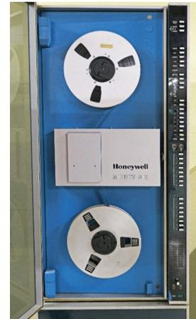
Fig 5: The Honeywell-96 Instrumentation tape recorder (front door opened, circuit compartment not shown)
