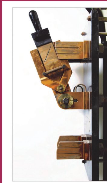
Figure 1. at the closing switch, the tension of the springs causes a quick separation of the contacts
