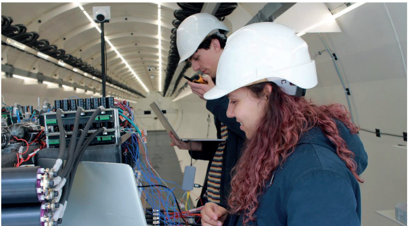
Figure 1. Testing the powertrain
