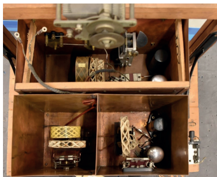
Figure 2 Top view of the generator (with panels removed)
