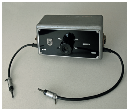
Figure 1. Amplifier GM 4574, giving an amplification of 100\times .
