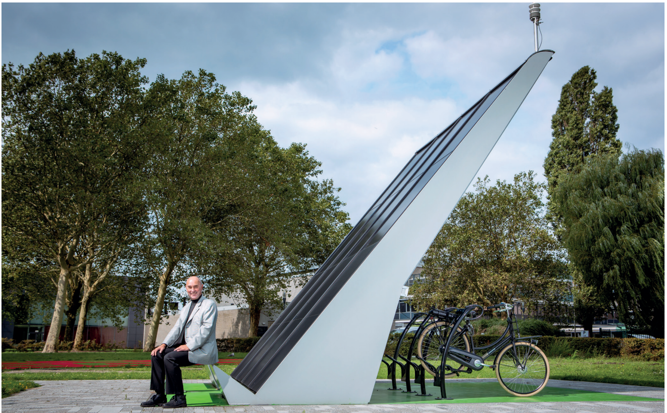
Figure 2. DC-operated prototype for charging bicycles, directly powered by solar electricity. It can be found next to EEMCS.
