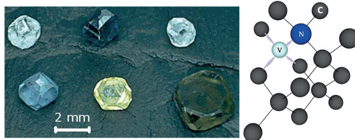
Figure 2. Colour centres in diamond are localized defects in the lattice structure created by the combination of vacancies and substitutional atoms (right, nitrogen-vacancy centre) and different impurity atoms give difference colours (left)
