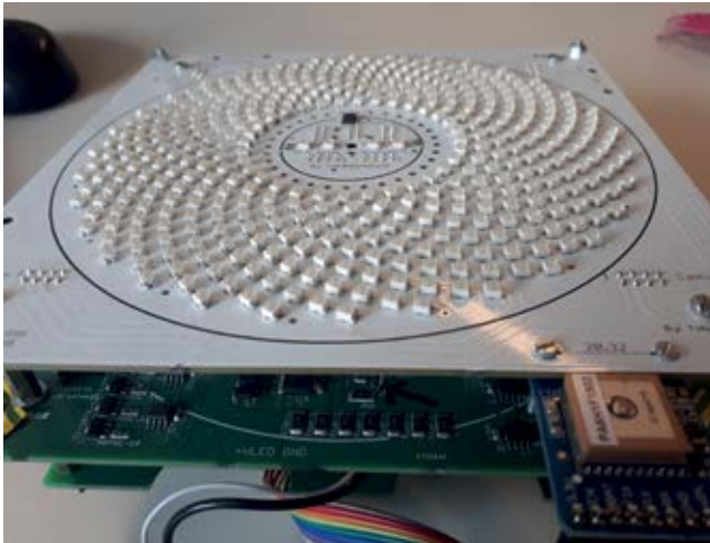
Figure 2. Inside a prototype infrared light
