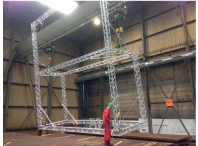
Figure 3. Real-size test setup for the camera system with an 8 x 8 m camera frame
