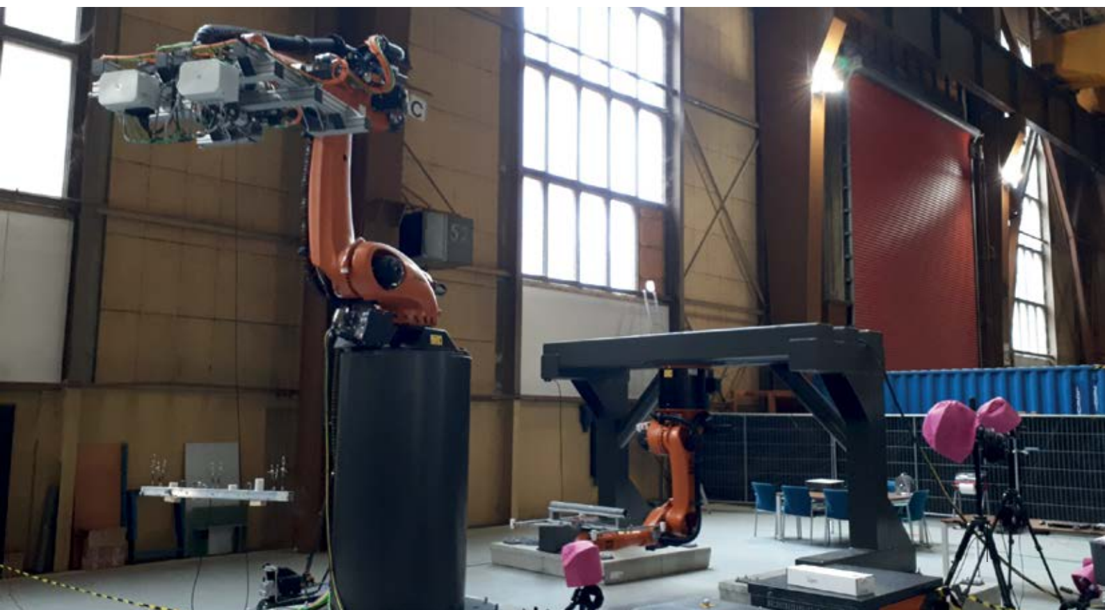
Figure 4. Scale 1:12 test setup for the motion controller
