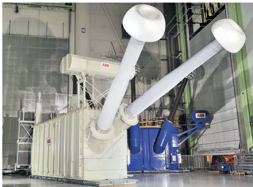
Figure 4. One of the 48 transformers of the 8000MW UHVDC Hami-Zhengzhou transmission link (source: ABB).
