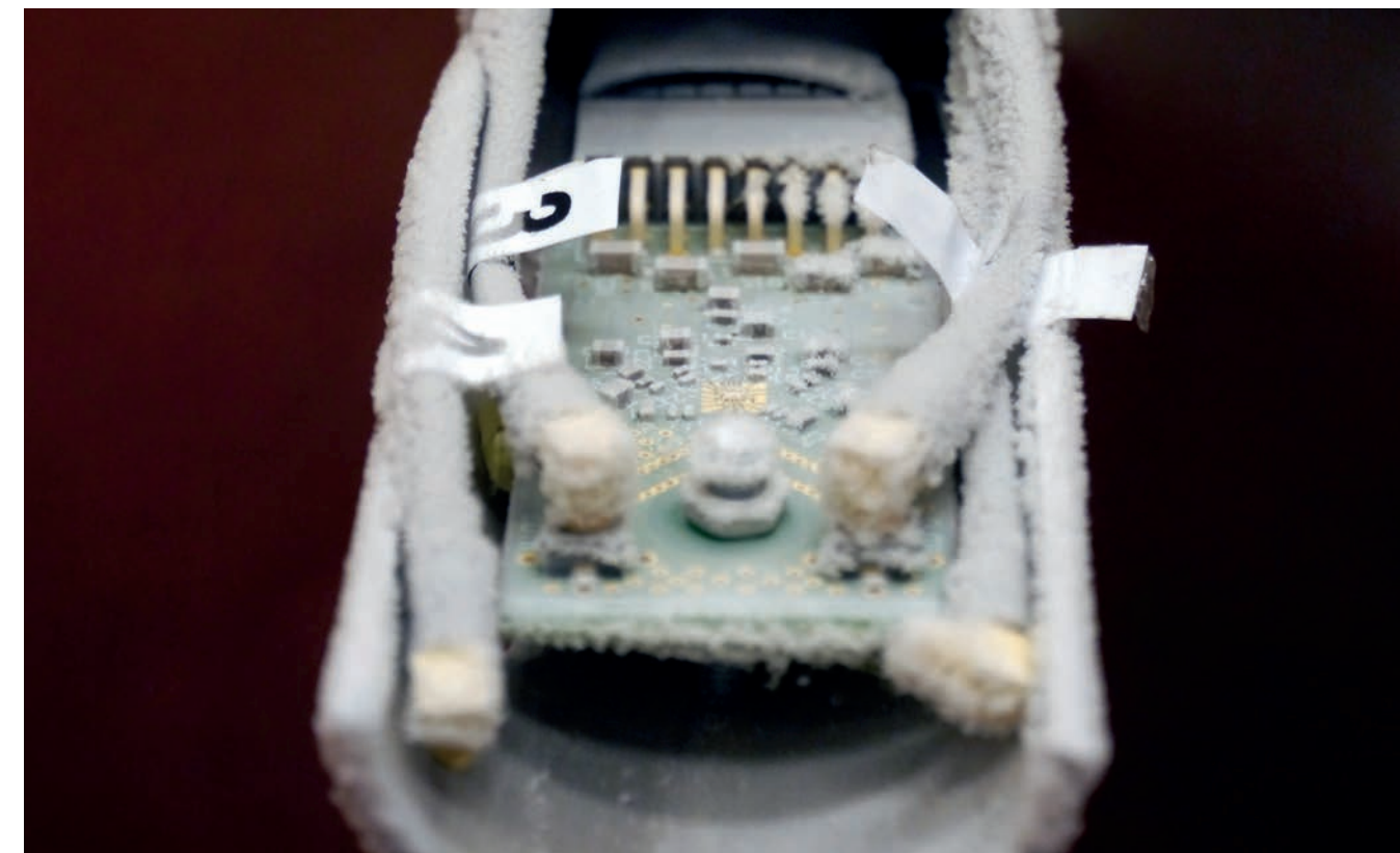
Figure 3. Cryo-CMOS chip (bonded on a PCB) just after a cool-down in liquid helium for cryogenic characterization.
