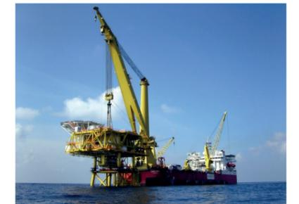
Figure 1. Huisman's off-shore installation, where EESS technology can be applied!
