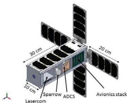
**Figure 3:** CAD external rendering of FLARE. Components from the +z face back include the lasercom payload, the Sparrow payload, ADCS, and avionics stack. Image credit: Derek Barnes, February 2017.
