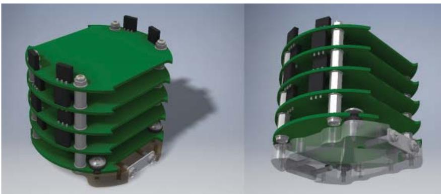
**Figure 3:** A render of the new modular electronics stack
