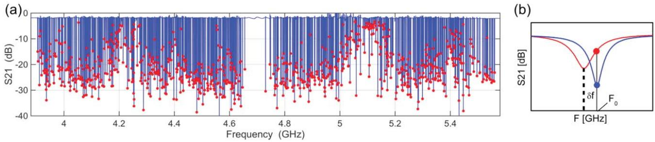
**Figure 2:** (a) Measured data of the transmission of the readout line of the chip shown in figure 1 at 0.12 K inside a test cryostat. Each dip corresponds to an individual pixel. (b) Response to radiation of a single pixel, reading out the pixel at a single frequency  $F_0$  will transform the measured change in resonance feature into a change in transmission at  $F_0$ .
