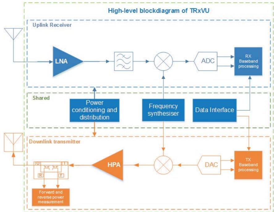
Figure 2: High-level block-diagram of TRXVU (source: ISIS)
