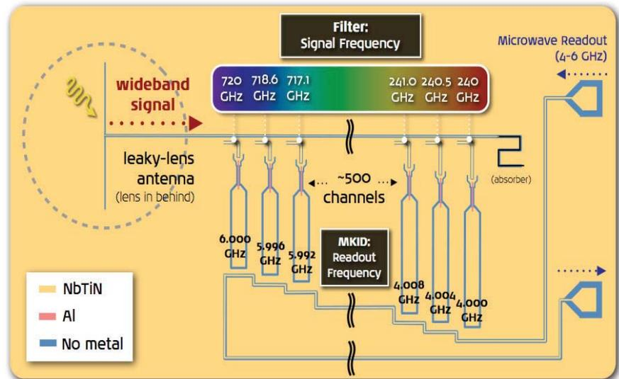
**Figure 1:** Conceptual drawing of the on-chip filterbank being developed for DESHIMA. The signal from the telescope, captured by a wideband antenna, is separated by a filterbank (an array of narrowband filters) and distributed to individual KID detectors. The entire filterbank will ultimately cover 240-720 GHz in a single shot with ~500 KID detectors.
