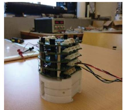
**Figure 4:** A prototype of the new modular electronics stack
