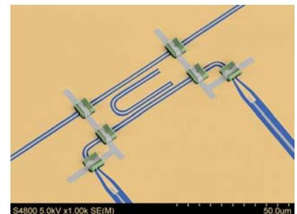
**Figure 2:** Scanning electron micrograph of a typical 350 GHz coplanar-waveguide filter of DESHIMA.
