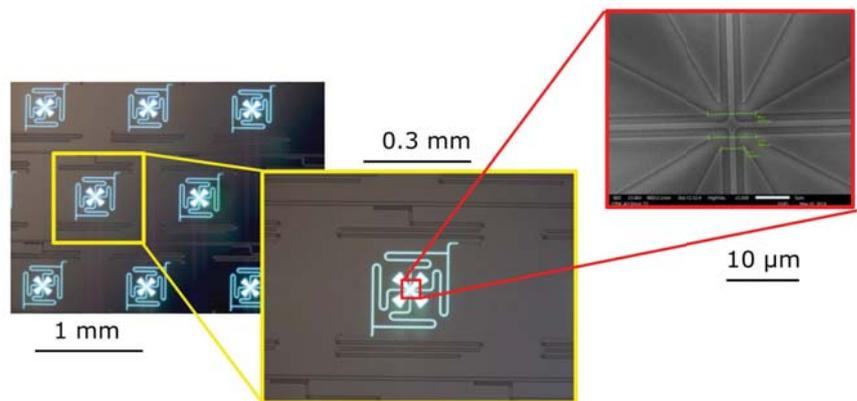
**Figure 4:** Small array of leaky-wave antenna coupled MKIDs. The image is made on an optical microscope with front and backlight. The antenna structure is made on a thin, transparent, membrane, the rest of the chip on a thick Si wafer. This highlights the antenna. The top right image shows a zoom, indicating the small feature size and cross CPW feed of the antenna.
