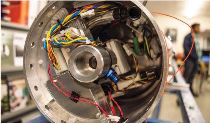
**Figure 2:** The Engine Bay of Stratos II+, including the valves and actuators
