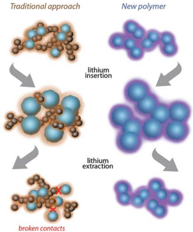
Figure 4: The principle of the old and new silicon anode
