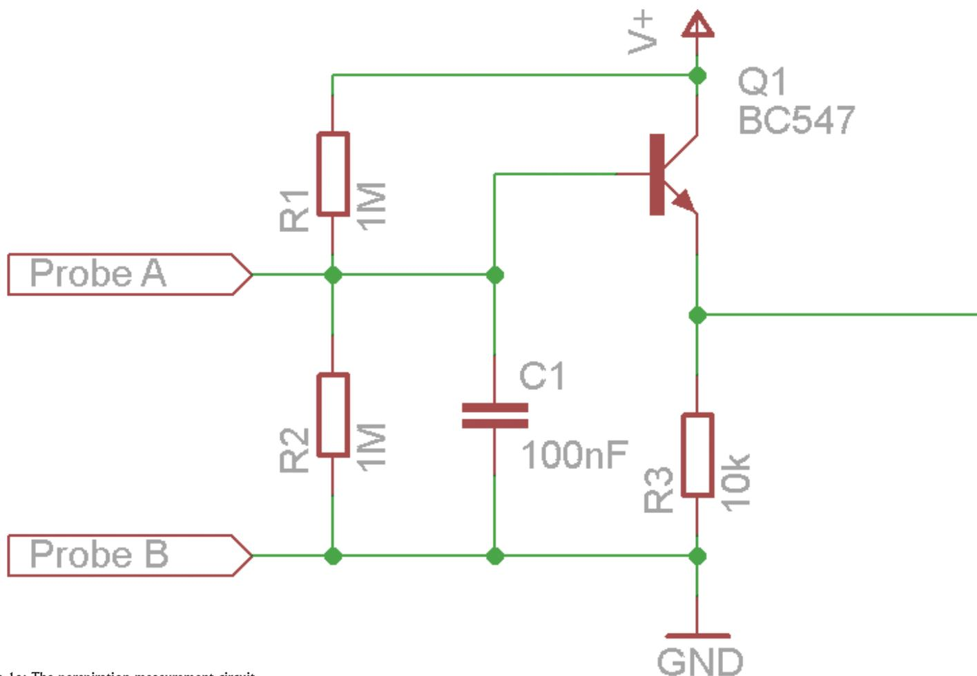
Figure 1a: The perspiration measurement circuit.
