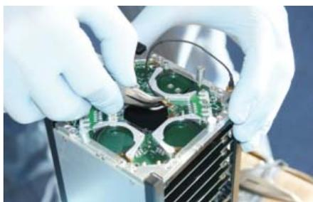
Connecting the deployable antenna system
