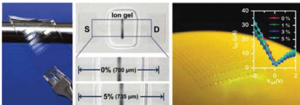
Figure 5: The flexible transistors (left, right) and their stretch performance (middle, right)
