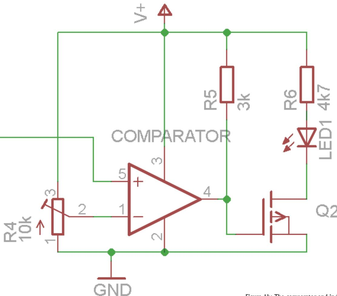
Figure 1b: The comparator and indicator circuit.
