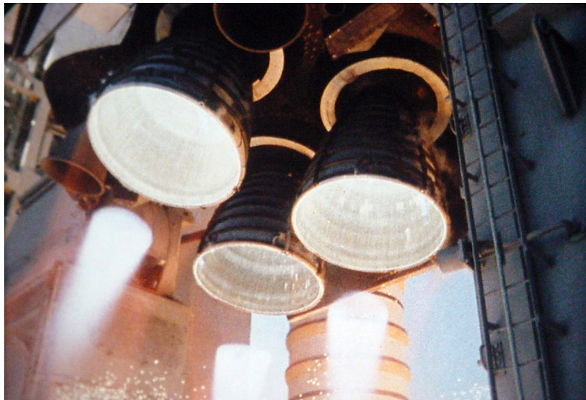
The main engines of the Space Shuttle. The pumps for each engine can empty a swimming
