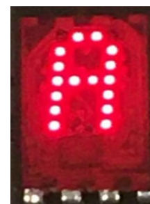
Figure 14. HP 5082-7340 4 by 7 led dot hexadecimal indicator (not to scale)
