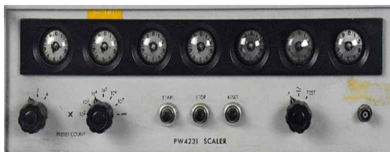
Figure 9. Philips Scaler 4231 using this special ZM 550 tube
