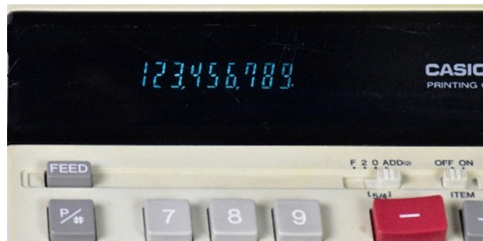
Figure 12. Casio FR 310 Printing Calculator using seven-segment indicators
