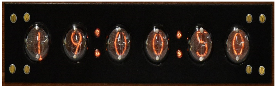
Figure 11. Electronic clock, which uses Nixie-tubes, displaying '19:00:50'
