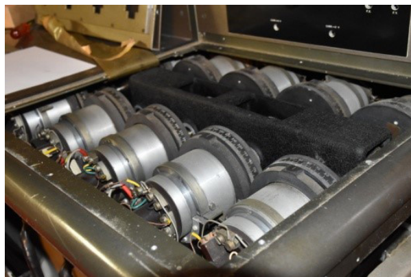
Fig 5. X-Y resolvers and the gear box. The positive resolvers rotate clockwise; the negative counter clockwise. The central resolver is stationary
