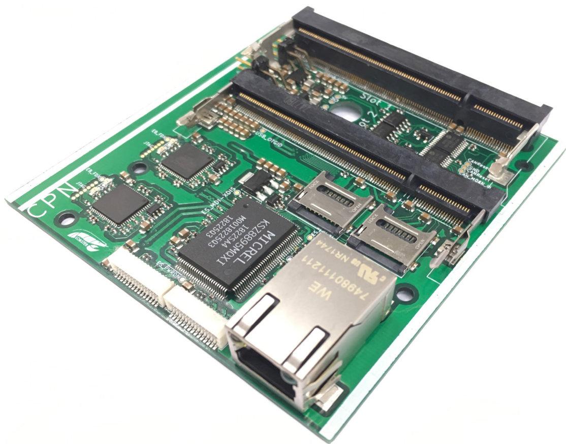
Figure 1. On-board computer module, hosting two Raspberry Pi's. Tested to work unto 400 bar
