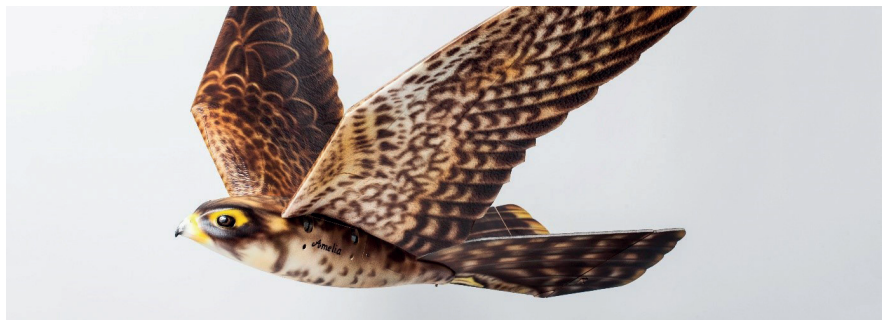
Figure 2. The Robird that has been developed at the University of Twente [1].
