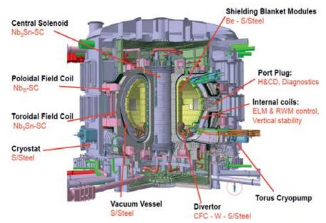
Figure 1. Schematic view of the machine (Courtesy of ITER organization).
