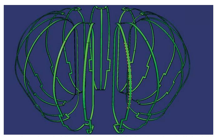
*Figure 3.* The green elements show 'cable trays' on the vacuum vessel, in the limited space between the vessel and the thermal shield. (Courtesy of ITER organization).
