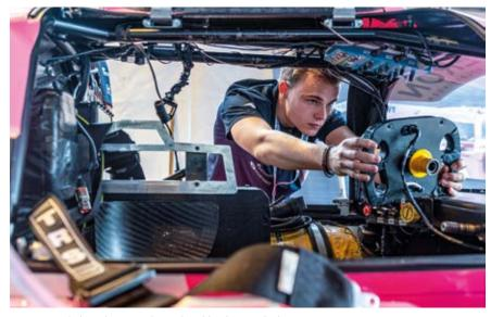
Figure 1. Fitting the steering wheel in the cockpit
