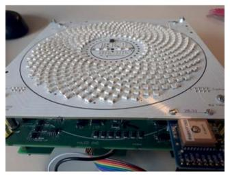
Figure 2. Inside a prototype infrared light
