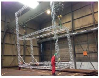
*Figure 3.* Real-size test setup for the camera system with an 8 x 8 m camera frame
