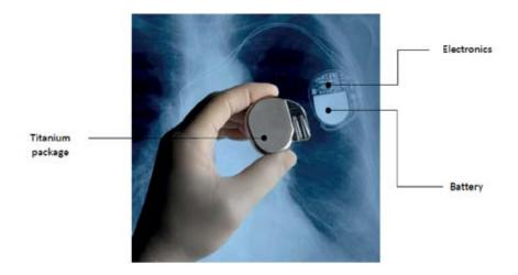
Figure 3. Conventional Ti packaging used for implants.<sup>[8]</sup>
