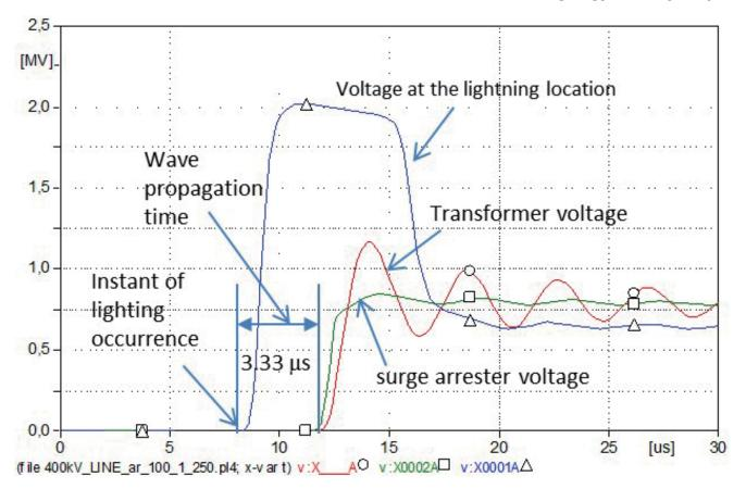
Figure 3. Voltage response at different location for a lightning impulse 1,2/50us, 10 kA
