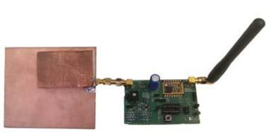
*Figure 3.* The PCB with the home-made antenna on the left side (for harvesting) and a transmitting antenna for LoRa on the right side.
