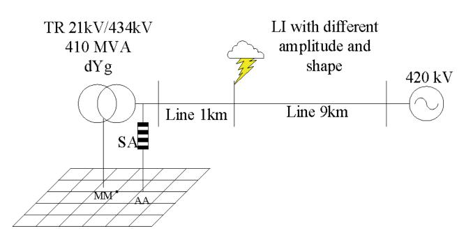
*Figure 2.* An illustration of a simulated system is shown. All components are modelled within a broad frequency range including the grounding system. The lighting occurs at a distance of 1 km from the substation.
