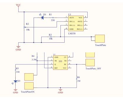
Figure 1. Touch button (top figure) and touch switch (bottom figure)
