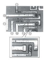
*Figure 2.* Corrosion of aluminium metal tracks in the presence of an electric field.<sup>[7]</sup>
