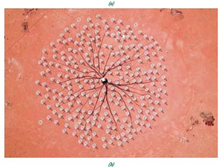
*Figure 3.* (a) A full station of 256 low-frequency antennas at the Murchison Radio-astronomy Observatory (MRO) in outback Western Australia, (b) top view (images courtesy of www.skatelescope.org)
