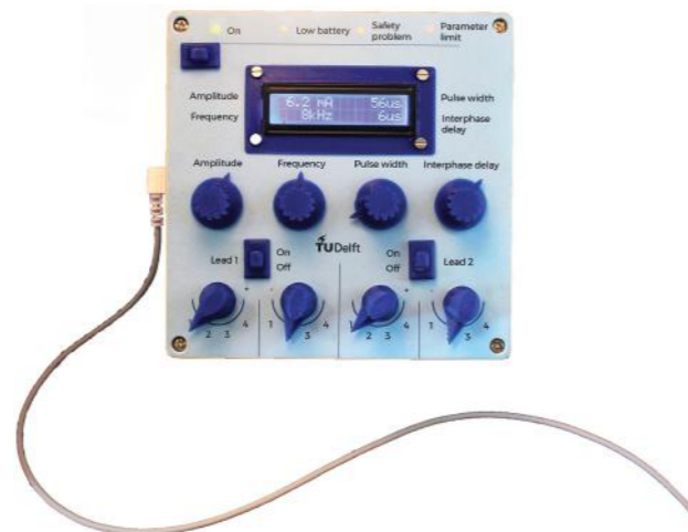
Figure 4. Our prototype with buttons to set the stimulation parameters which can be viewed on the LED screen.
