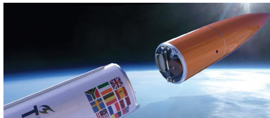
Figure 5. Separation is one the most crucial phases during the mission and relies on firing bolt cutters in a spring-loaded mechanism. Altitude detection must be on point as well as the timing of the parachute deployments that follow on the way down.
