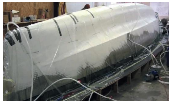
Figure 3. Resin being transferred to a sailboat hull [9].
