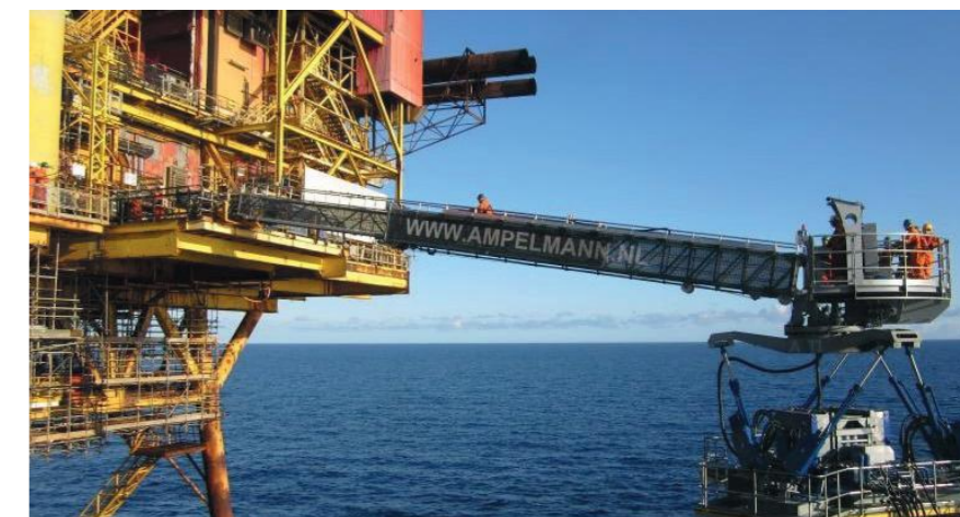
Figure 1. An Ampelmann system in 'engaged' mode, allowing safe transfer from ship to offshore structure.
