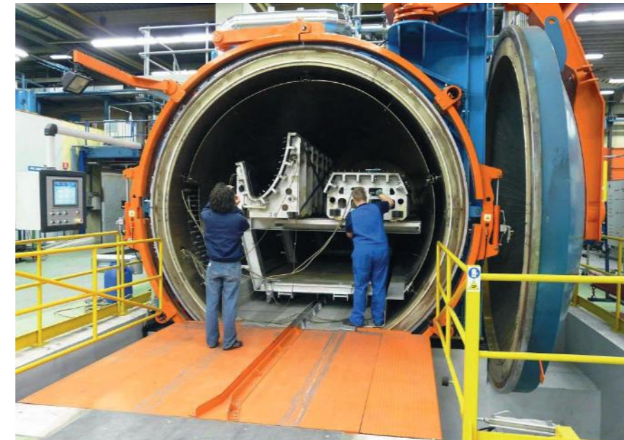
Figure 4. Parts being cured in an autoclave [10].
