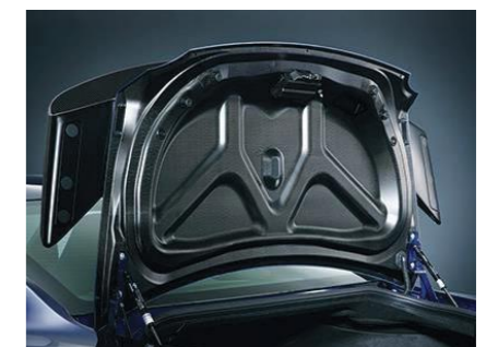
Figure 6. Compression molded Nissan GT-R decklid [12].
