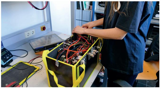
Figure 2. Energy Box of the TU Delft Solar Boat.
