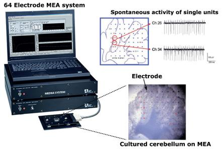
Figure 2. Typical commercial MEA recording system. Adapted from www.med64.com.
