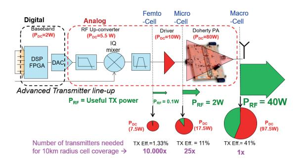
Figure 2. Typical analog intensive high-end macro-cell base station line-up. Note that when truncating the transmitter chain at a lower power level, for example, to address the needs of a smaller cell base station, the required DC power becomes lower, but also the related system efficiency, while more base station nodes are needed to cover a similar geographic area.
