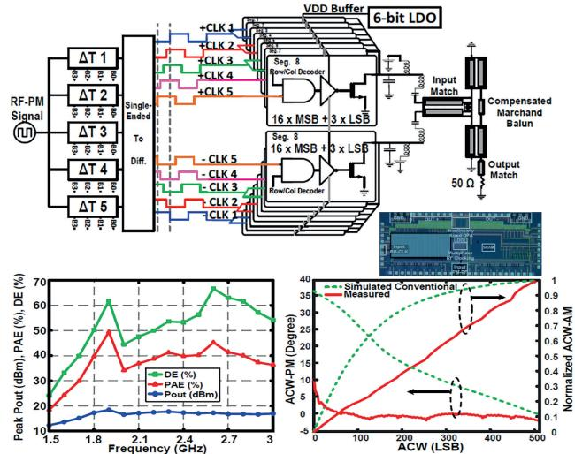
Figure 3. New digital intensive Polar Transmitter architecture using non-uniform segmentation, overdrive control and multi-phase clocking of the (segmented) final transistor stage. This yields an intrinsically linear conversion of the binary amplitude code word (ACW) to RF output amplitude (AM) and phase (PM), as can be seen from the ACW-to-AM and ACW-to-PM transfer functions, the realized circuit can provide signals with up to -50 dBc ACPR without using any pre-distortion.
