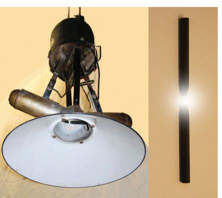
Figure 1. An electric arc lamp and two carbon rods as present in the historic collection of the Faculty EEMCS (photo: Han Geijp).
