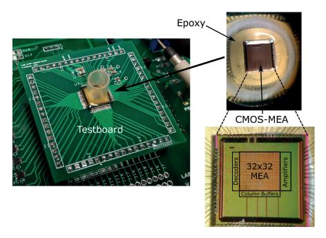
Figure 3. Example of a 32X32 CMOS-MEA chip that can perform both EIS and CS depending on the application. Each sensor is 15x15 µm<sup>2</sup> and the chip measures 10 mm<sup>2</sup> [Adapted from Valente et al. Manuscript in preparation].
