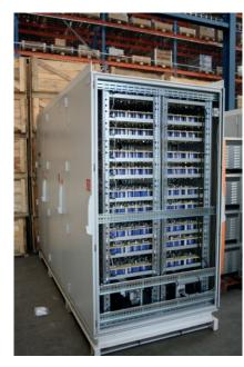
Figure 1. Super capacitor-based energy storage
