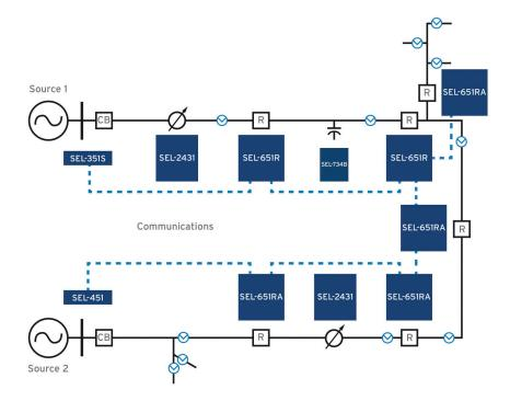
Figure 4. SEL Distribution Network Automation [14].
