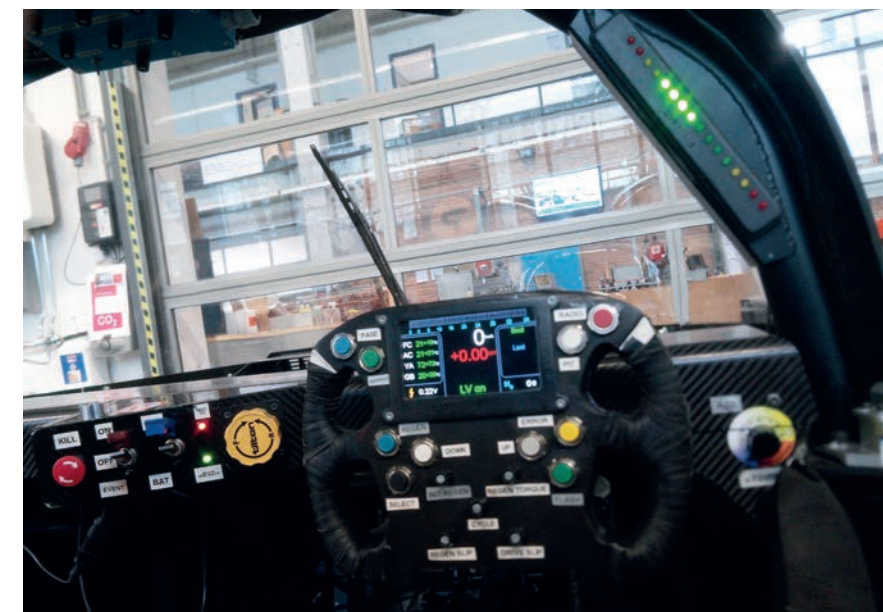
Figure 1. Dashboard of Forze VII with a driver interface on the steering wheel.
