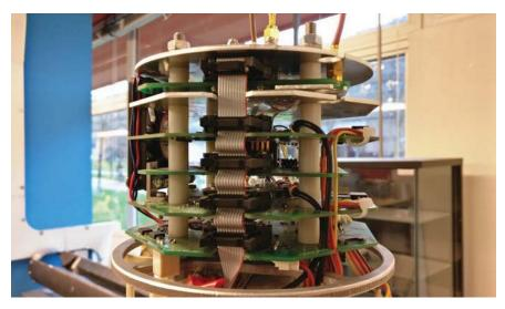
Figure 1: The main Electronics Stack of the Stratos II+ mission
