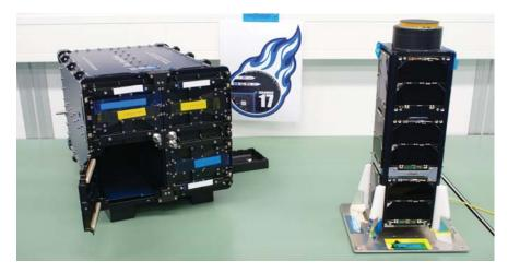
Figure 4: Did0-2 CubeSat (right) and its orbital deployer (left)
