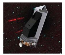
**Figure 3:** Artist's rendition of the proposed NEOCam space telescope, which would survey the regions of space closest to the Earth's orbit, where potentially hazardous asteroids are most likely to be found. Credit: NASA/JPL-Caltech
