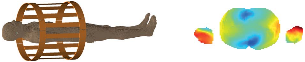
Figure 3: On the left side a typical simulation configuration, created with Remcom XFDTD software. The birdcage antenna around the human voxel model emits the RF field. The right figure depicts the B_1^+ field for a transverse slice around the liver. The signal voids (blue) are clearly visible in the anterior and posterior.
