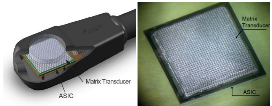
Figure 3: Miniature ultrasound probe for cardiac imaging from the esophagus: (left) an artist’s impression of the probe; (right) a realized prototype chip with a 1024-element matrix transducer built on top.
