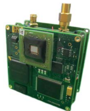
Figure 4: The FluoCAM camera system consists of three PCB, containing the camera module, FPGA, delaylines and voltage regulators [5].
