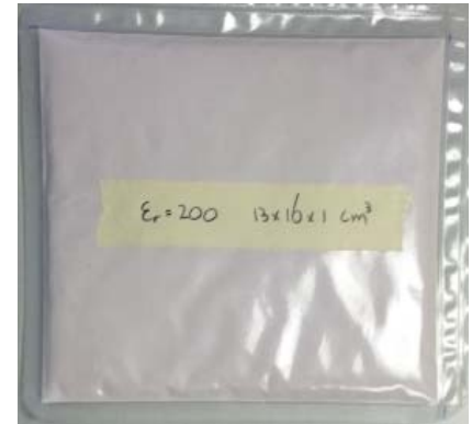
Figure 2: High permittivity pad with a relative permittivity of 200 and dimensions 13x16x1 cm 3 . The material of the pad is a mixture of calcium titanate, barium titanate, and deuterated water.
