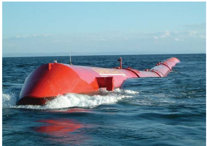
Figure 4: Pelamis Prototype (attenuators)
