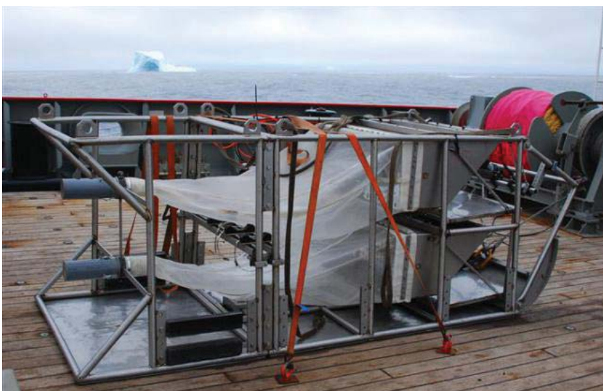
Figure 4: The Epi-Benthic Sledge, complete with compulsory iceberg
