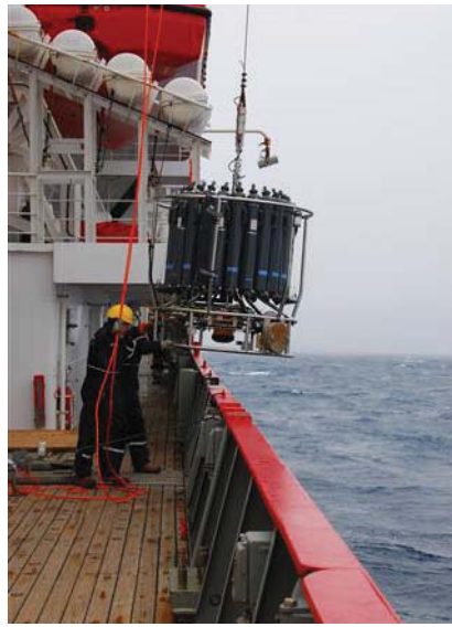
Figure 1: Deploying the CTD
