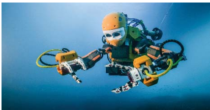
Figure 2: A new humanoid robotic diver from Stanford, explores a 17th century shipwreck. (Image credit: Frederic Osada and Teddy Seguin/DRASSM)
