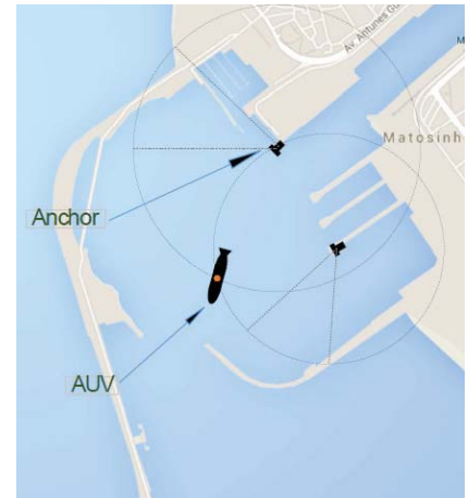
Figure 4: Underwater localization of UAVs using only two fixed anchors (Porto harbour, NOPTILUS project)
