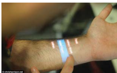
Figure 1: The Skinput-system projecting buttons on an arm.
