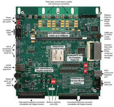
Figure 11: The Xilinx FPGA board that was used
