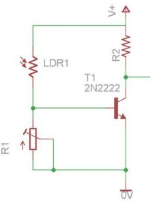
Figure 2: LDR sensor and surrounding circuitry
