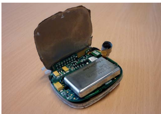
Figure 3: The inner workings of a neural stimulator.
