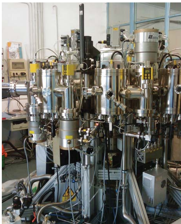
Figure 3: Amigo machine for the deposition of silicon films installed at Dimes
