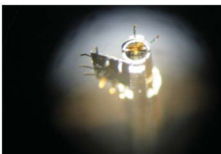
Figures 3&4. The circuit is put in the head of the guidewire, and folded around soon after
