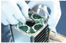
Connecting the deployable antenna system
