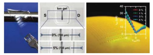
Figure 5: The flexible transistors (left, right) and their stretch performance (middle, right)
