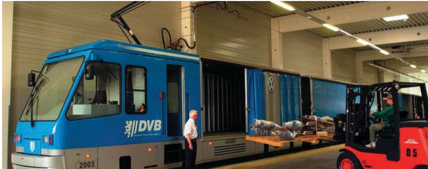
The tram is actually the Volkswagen tram that brings parts from the logistics facility to the Transparent Factory. It looks quite a bit like a normal Dresden tram-car, but if you look at the side of it, you can see that it is a 'freighter', not a passenger tram.
