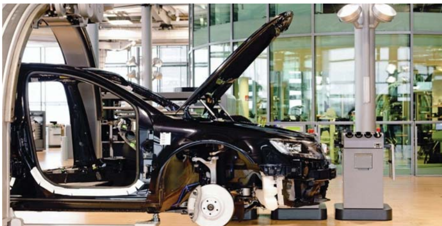
A Klavierlack Black Phaeton, quite early in the build process. Some components have been installed, but work on the interior trim and running gear has not started.
