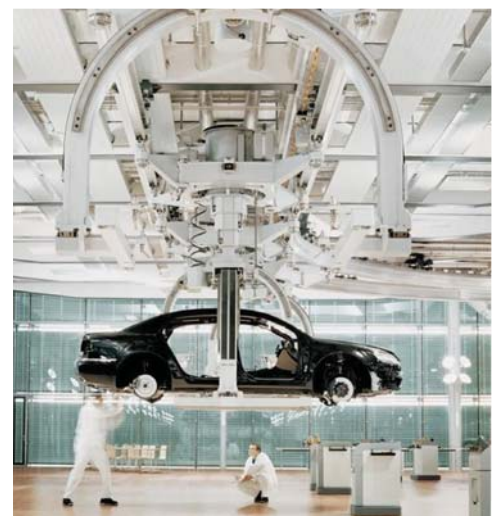
Once the Phaeton is on the overhead crane assembly, it is left there until all the required work on the underside of the car has been completed.
