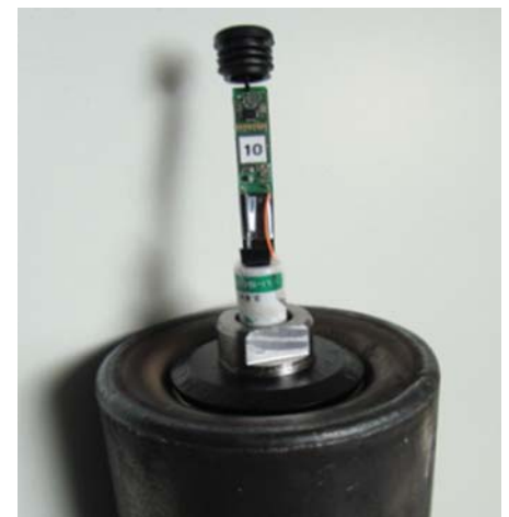
Figure 6. Idler roll with embedded sensor
