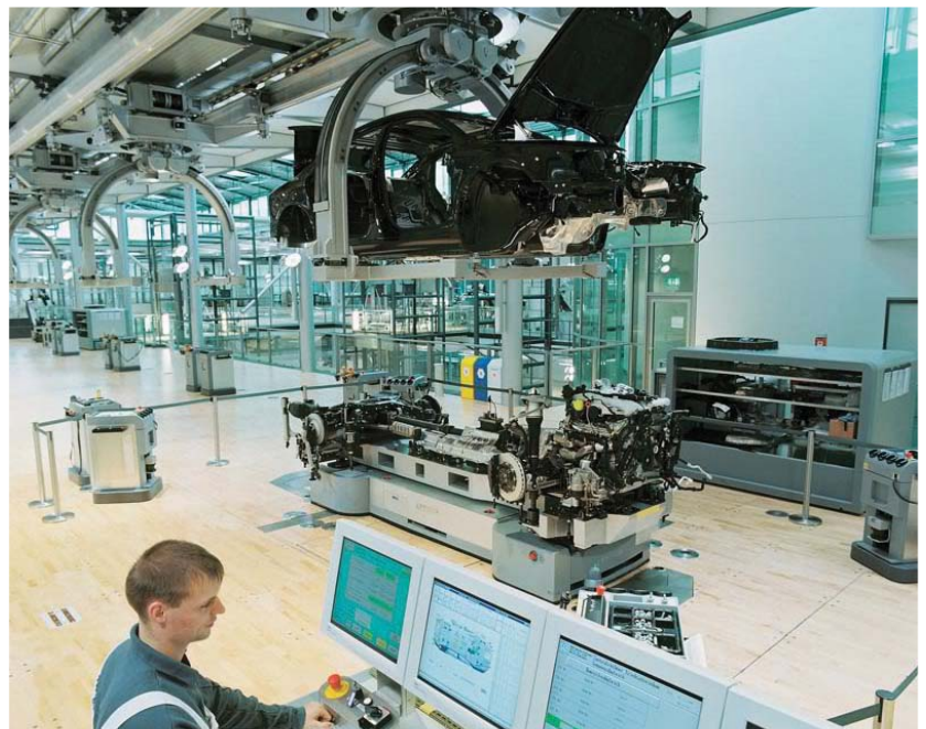
Once all the wiring and electronic components are installed into the carrosserie, it is then time to mate the body-structure with the running gear. The running gear is also assembled by hand, and brought to the main production area by an elevator.
