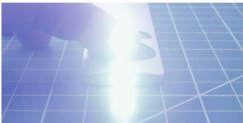
Figure 4: Apple IR remote photographed using a digital camera. Though the emitter is quite bright and the frequency emitted is not far past the red portion of the visible spectrum, it's completely invisible to the eye.
