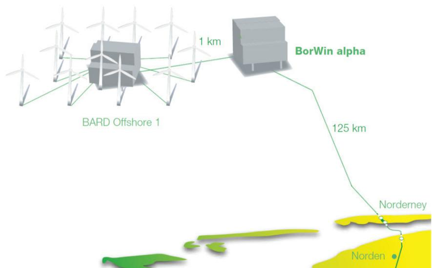
**Figure 3.** BorWin Alpha converter platform configuration (courtesy of TenneT)
