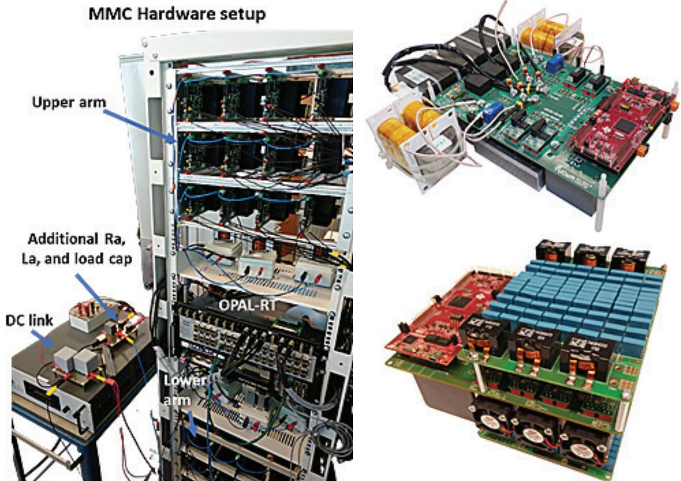
{Order: Clockwise} **Figure 1:** (a) Downscaled modular multilevel converter for MV DC-distribution grids; EV battery chargers (b) 11 kW DC-type EV charger based on a versatile phase-shift forward converter with voltage- or current-doubling functionality; and (c) 7.7 kW wireless charging converter based on the LCC resonant converter (primary-side power electronics shown only).
