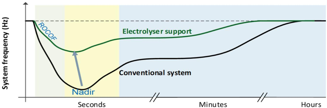
Figure 5. Contribution of electrolyser to frequency stability: limiting the frequency deviation Power lab.)
