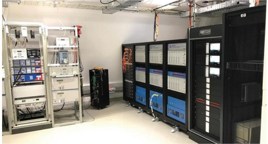
Figure 4. Real Time Digital Simulator in the TU Delft Electrical Sustainable Power lab.)
