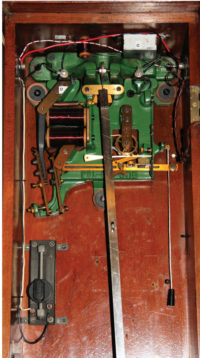
**Figure 2.** A gravity arm driven pendulum of a PUL-SYN-ETIC master clock, built by GENT of LEICESTER (1938)
