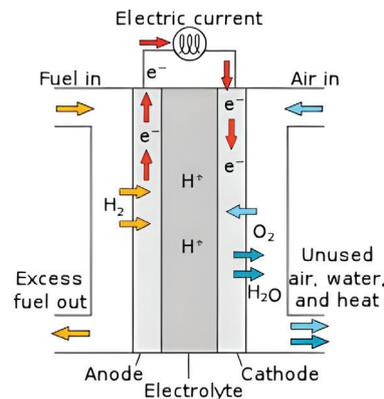
**Figure 2.** Working of a fuel-cell
