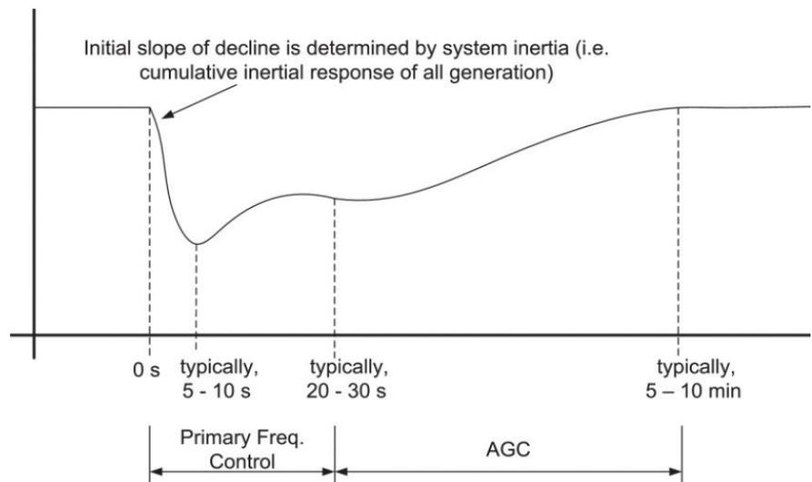
**Figure 2.** An illustration of power system frequency response to a major loss of generation. (reproduced from [1] and [2])
