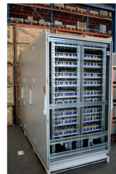
Figure 1. Super capacitor-based energy storage.
