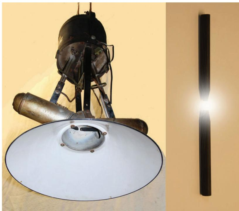
Figure 1. An electric arc lamp and two carbon rods as present in the historic collection of the Faculty EEMCS (photo: Han Geijp).
