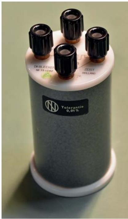
**Figure 2:** Precision resistor by C. Bleeker, Zeist (Photo by: Kees Pronk)
