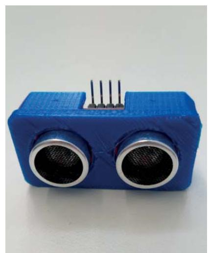
**Figure 3:** An ultrasonic obstacle detection sensor in its 3D printed encasing
