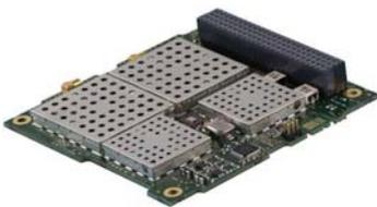
**Figure 3:** ISIS VHF uplink/UHF downlink Full Duplex Transceiver
