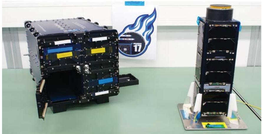
**Figure 4:** Did0-2 CubeSat (right) and its orbital deployer (left)
