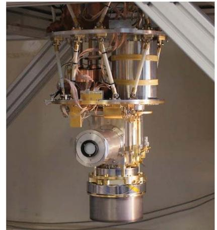
**Figure 4:** Photograph of the DESHIMA cryogenic optics, housing the 100 mK stage on which the filterbank chip is mounted.
