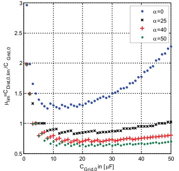
Figure 10:  $\mu_{lim}$  as a function of  $C_{Grid,0}$  for a feeder cable length of 10km and  $\mu=0, 25, 40$  and  $50$
