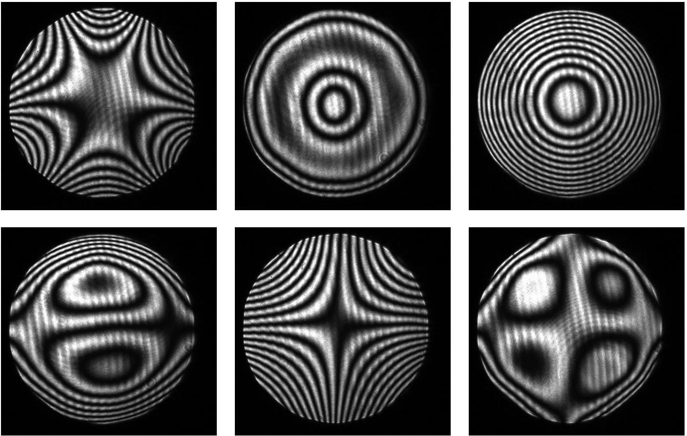
Figure 1: Interference patterns are used to measure the deformation of mirrors. A perfect spherical mirror should have a number of concentric circles.
