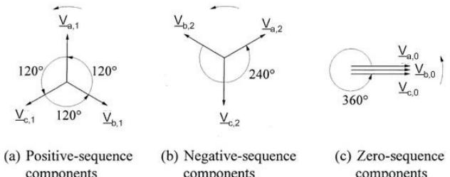
Figure 2: Sequence components during system unbalance
