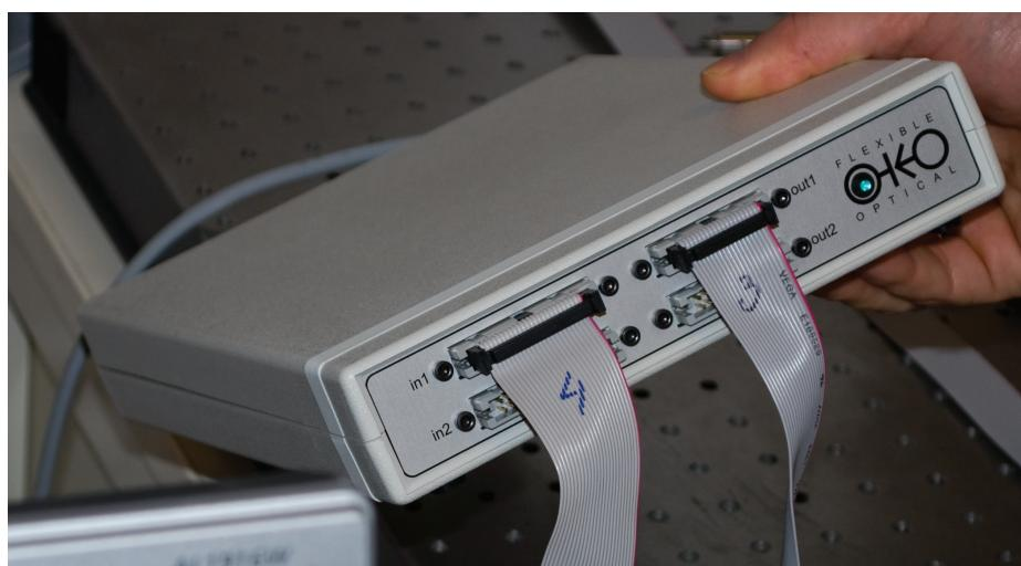
Figure 3: A box that can control up to 40 actuators
