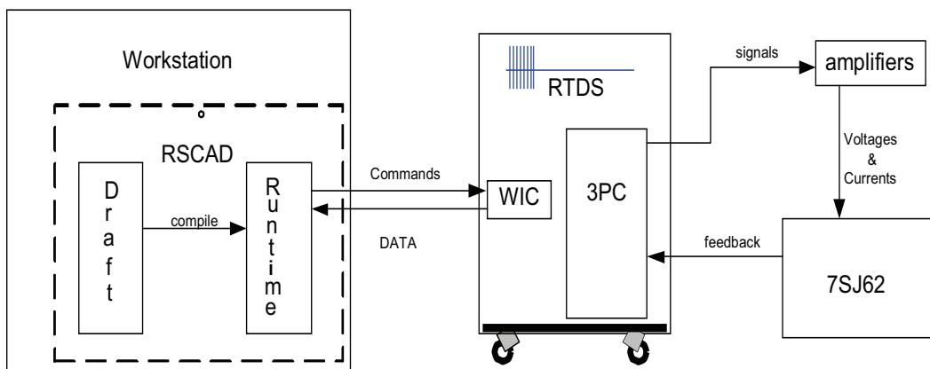
Figure 11: Closed-loop operation of protection equipment and RTDS.
