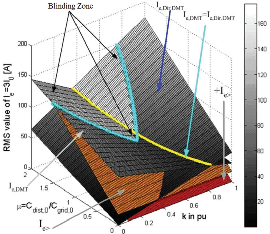
Figure 9: Presence of a blinding zone during a single phase-to-ground fault in cable 2 as the fault location  $k$  and the network capacitance factor  $\mu$  are varied. Earth-fault currents measured at both cable ends are depicted as two planes crossing each other at the indicated line.  $I_{e,>}$  and  $+I_{e,>}$  are DMT2 and Dir.DMT2 settings respectively, which vary with  $\mu$  as well, spanning two parallel planes.
