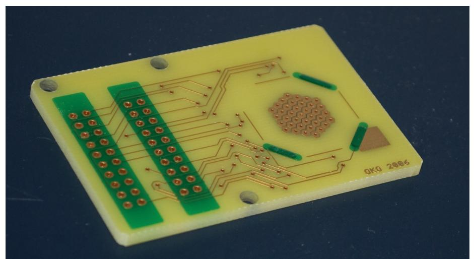
Figure 2: A PCB on which a flexible mirror can be attached. This PCB supports 37 actuators.
