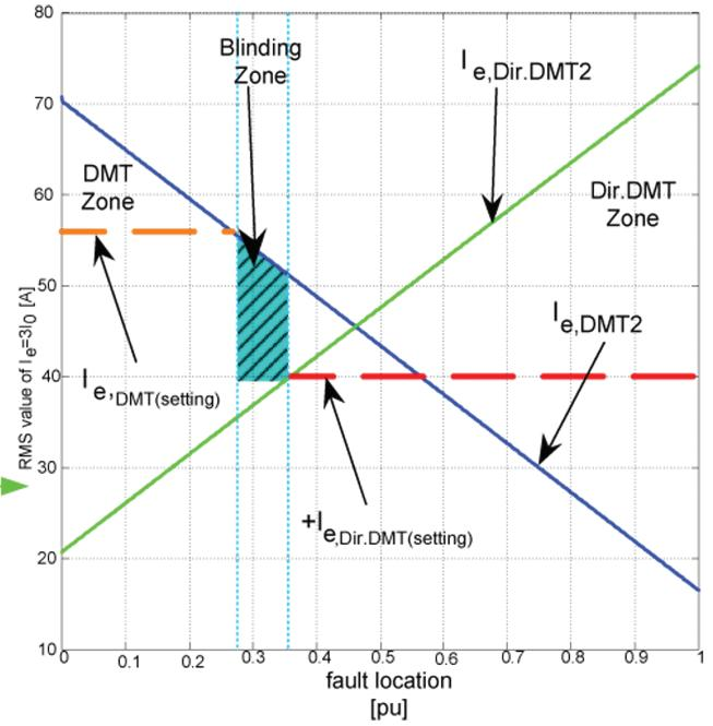
Figure 8: The presence of a blinding zone in the encircled part of the network. For a certain range of the fault location  $k$ , the fault currents from both sides are too small for the relays to respond. The orange dashed line represents the  $I_{e,DMT}$  setting while the red dashed line represents the  $+I_{e,Dir.DMT}$  setting.  $k$  can be varied from 0 (node p) to 1 (node q).
