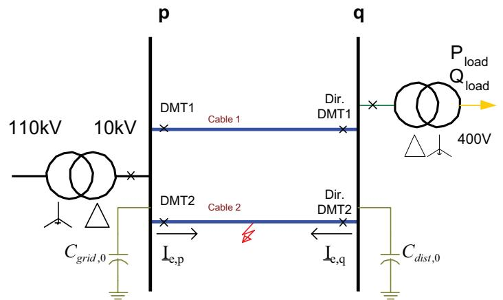
Figure 6: Simplified network used for earth-fault analysis
