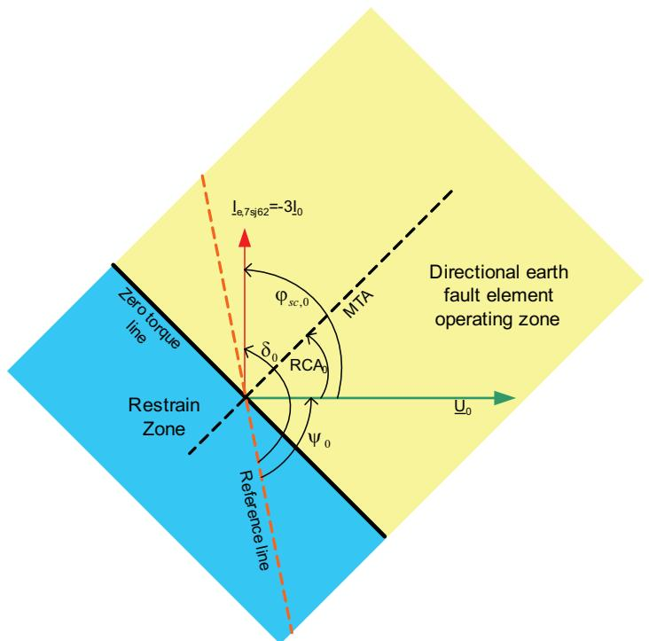
Figure 7: Phasor diagram of a typical directional earth-fault element. Zero-sequence voltage  $U_0$  is used as a reference phasor for direction determination.  $RCA_0$  of  $45^\circ$  is applied.
