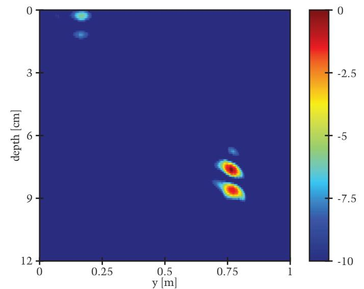
Figure 7: Deconvolution result of sub-surface landmine [dB]
