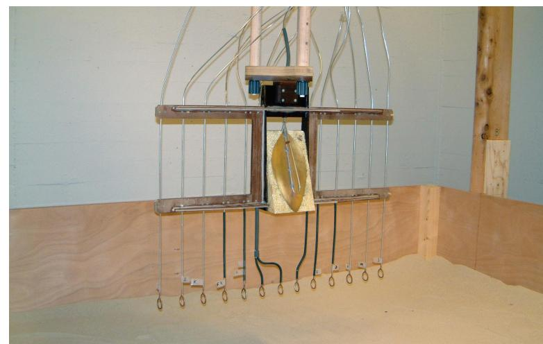
Figure 1: Array of 13 receiving antenna loops
