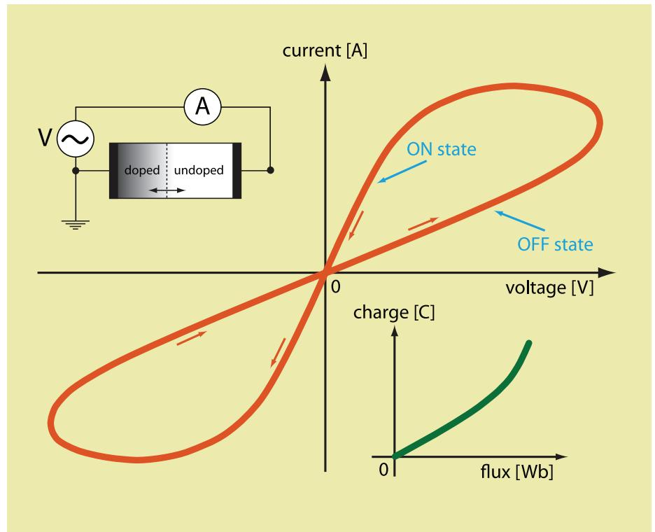
Figure 2: Current-voltage plot demonstrating hysteretic phenomena of HP Lab's memristor. The application of a sinusoidal voltage ( $V$ ) across the device will move the boundary between the doped and undoped regions causing the charged dopants to drift. The distribution of the dopants, and thus the resistance of the device, is proportional to the charge that passes through. Note the corresponding charge-flux plot shows a much simpler non-hysteretic relationships.
