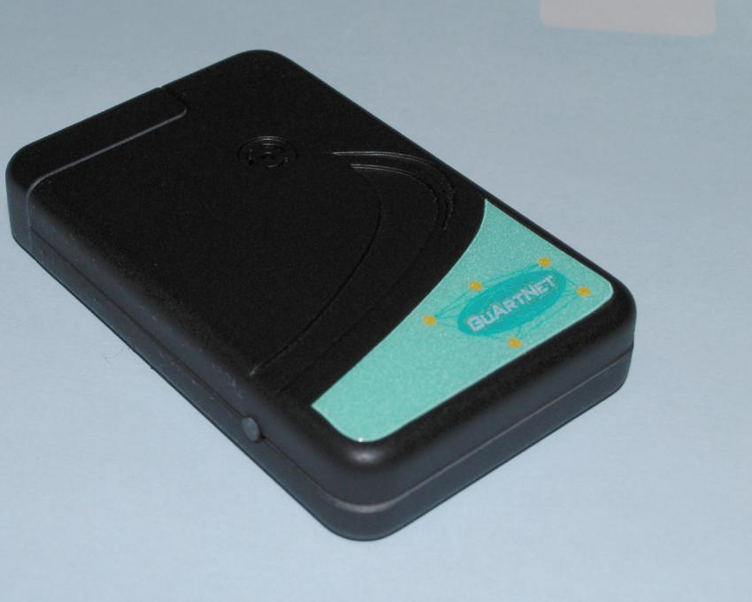
The museum sensor. Inside are a.o. an L-Node, a vibration sensor, and two AA batteries.
