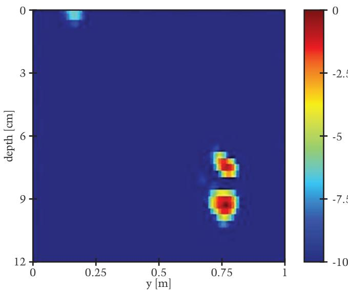
Figure 6: Diffraction stack result of sub-surface landmine [dB]
