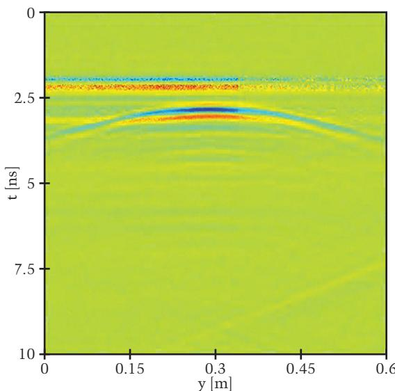
Figure 3: Original B-scan (signal level)
