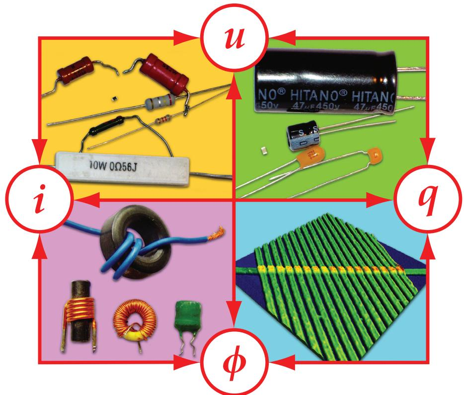
Figure 1: The four element quadrangle. An inductor corresponds to a static relationship between current  $i$  and flux  $\phi$ , a capacitor corresponds to a static relationship between voltage  $u$  and charge  $q$ , and a resistive element corresponds to a static relationship between current and voltage. There are two dynamical relationships, one between current and charge, and the other between voltage and flux. The remaining relationship, namely between flux and charge, defines a memristor.
