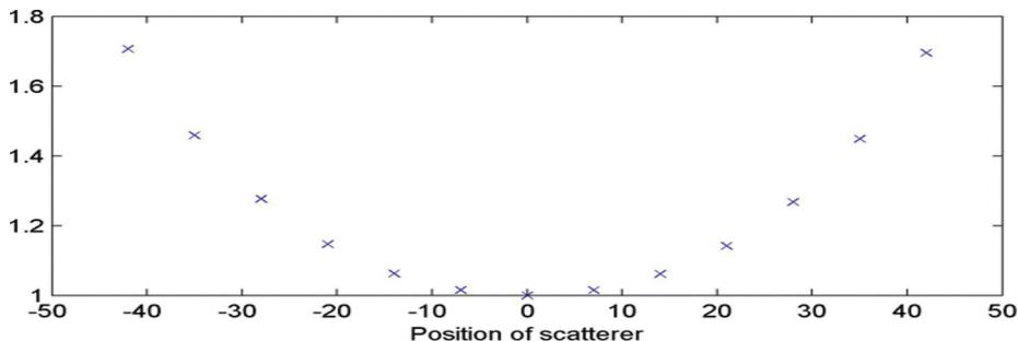
Figure 11: Weights for each deconvolution result related to position of scatterer
