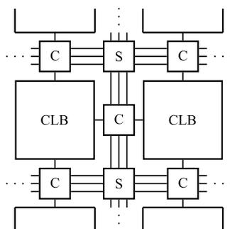
Figure 6: FPGA Layout
