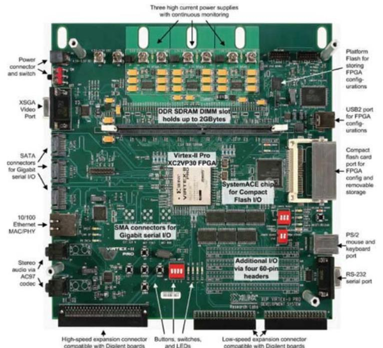
Figure 11: The Xilinx FPGA board that was used
