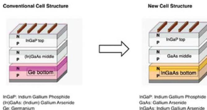
Illustration of Sharp's new solar cell structure
