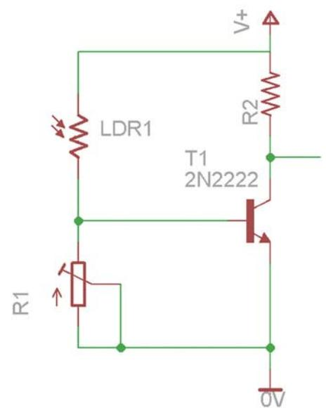
Figure 2: LDR sensor and surrounding circuitry
