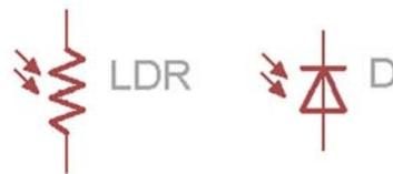
Figure 1: Symbols for an LDR and photodiode
