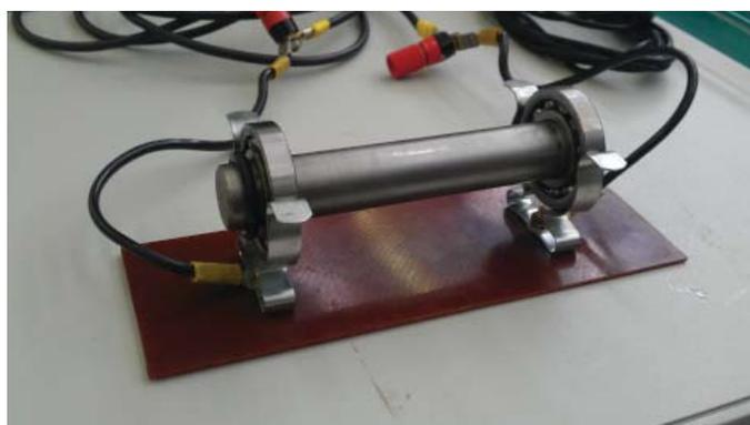
Figure 1: The ball bearing engine
