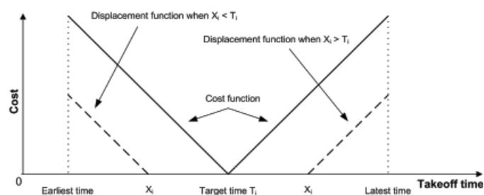
Figure 2: Cost function for an individual aircraft
