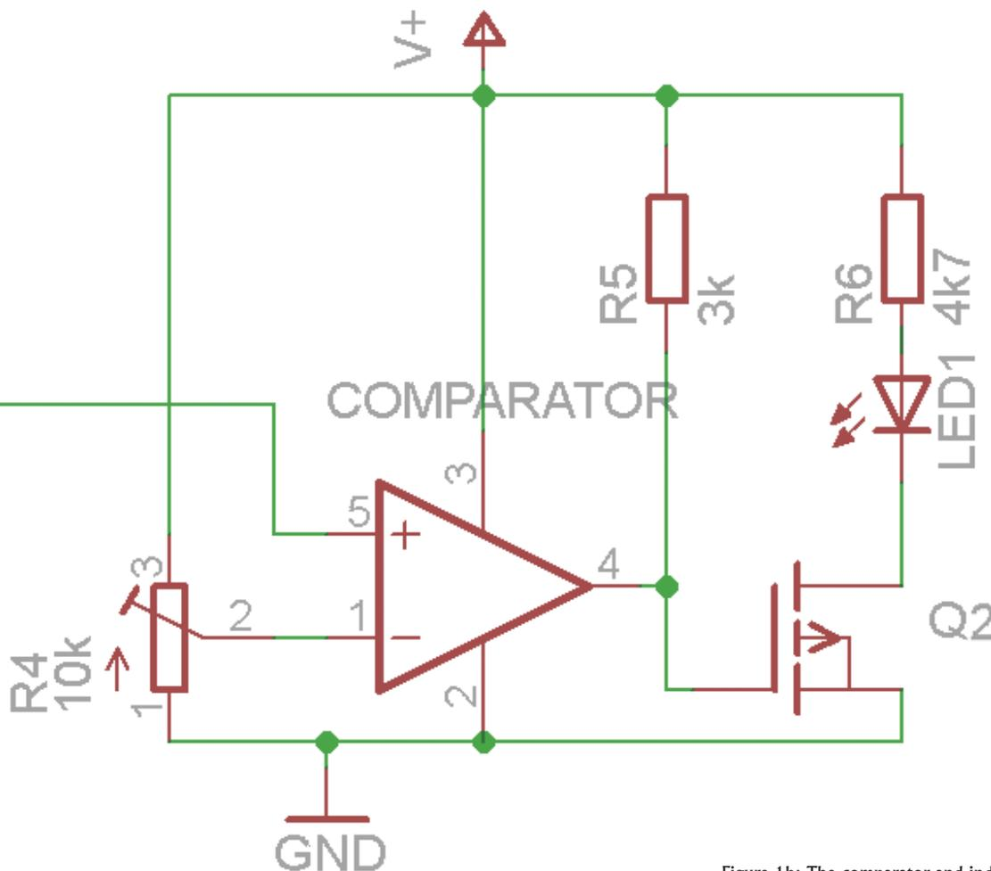
Figure 1b: The comparator and indicator circuit.
