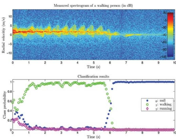
Figure 2. Measured spectrogram for a walking human and its classification results
