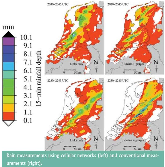
Rain measurements using cellular networks (left) and conventional measurements (right).
