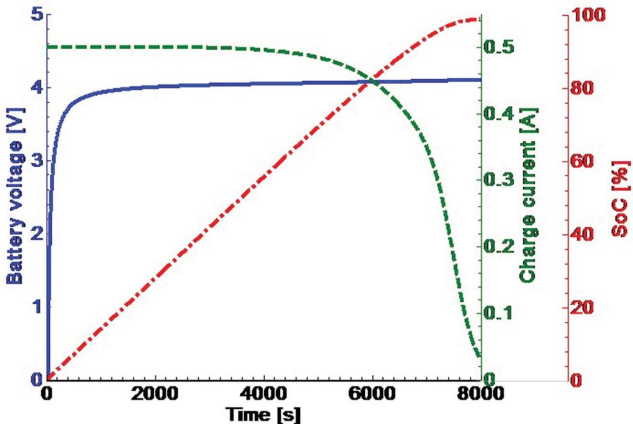
Figure 1: Hyperbolic tangent charge curve. Blue solid line indicates battery voltage rise over charge time. Green dashed line indicates charge current decay over charge time. Red dash-dotted line indicated rise of the battery State of Charge (SoC). Note that the charge current decays in a hyperbolic tangent manner as soon as the battery voltage is close to the final charge voltage.
