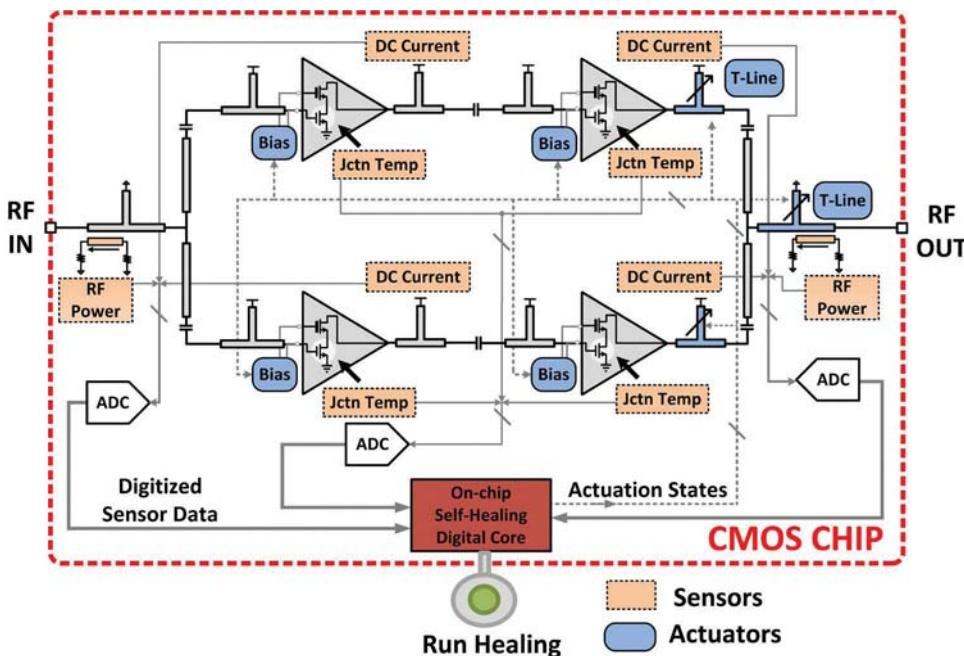
Schematic of the self-healing chip design
