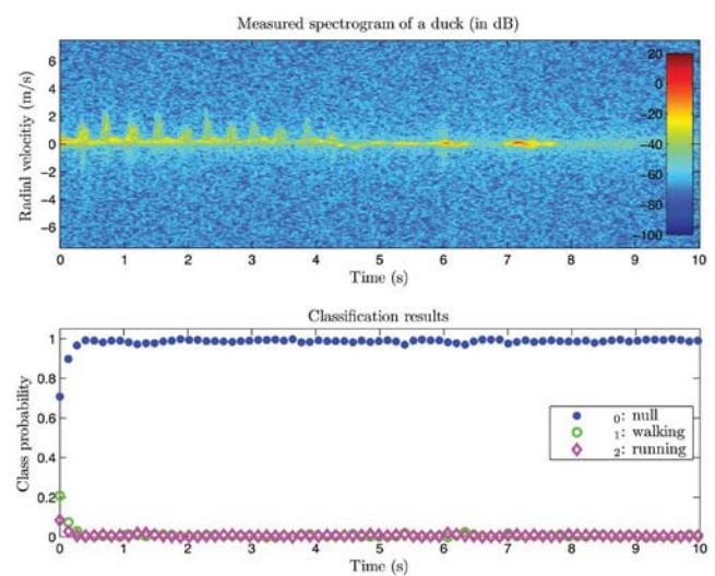
Figure 4. Measured spectrogram of a duck and its classification results
